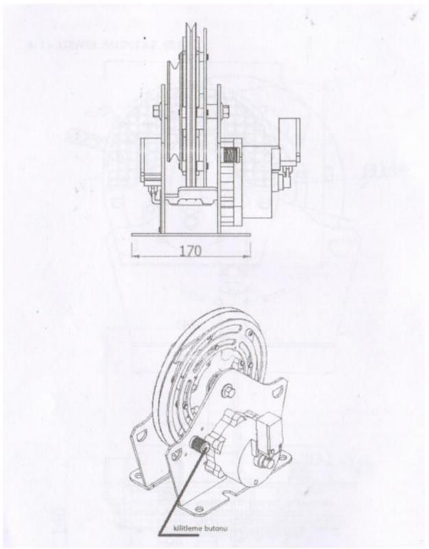
Locking button: It is used in low speed brake tests. The governor is locked by pressing this button while the elevator is in action. During this process, the button should be pressed continuously until brake locking emerges.
